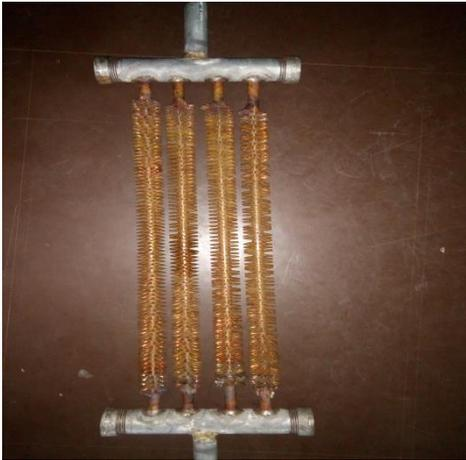
Fig. 4. Advanced designed finned Copper tube
