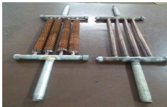
Fig. 3. Copper Tubes as Heat exchangers
