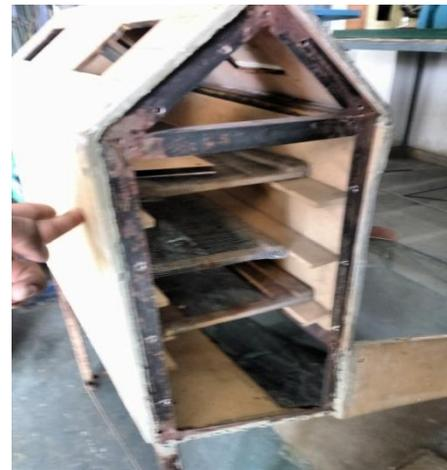
Fig. 4. Arrangement of the trays in cabin before drying
