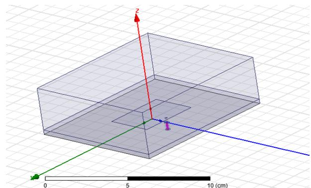
Fig. 2.1. Design of Coaxial Feed antenna
