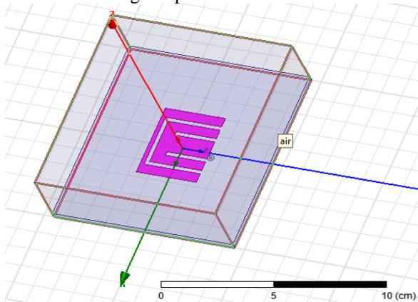
Fig. 3.2. EU Microstrip Patch Antenna
