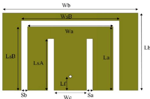
Fig. 3.1. Design of EU shaped patch antenna
