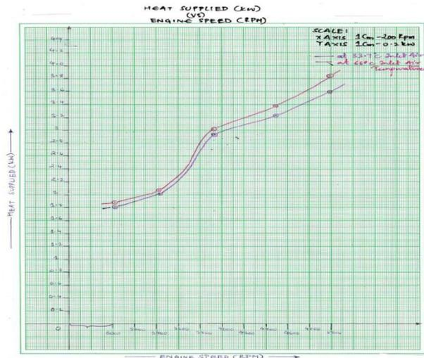
Graph: Engine speed vs heat supplied efficiency
