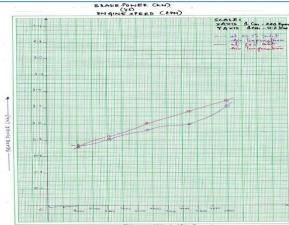
Graph: Engine Speed Vs Brake power
