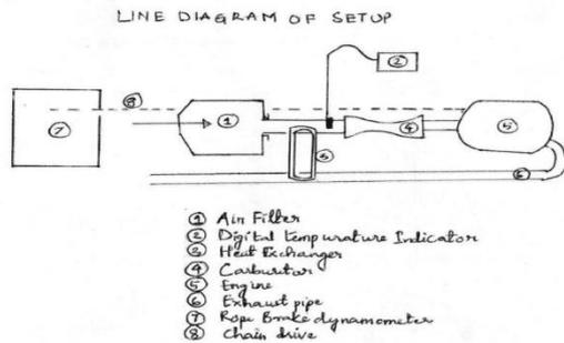
Fig. 4. Schematic layout of Experiment
