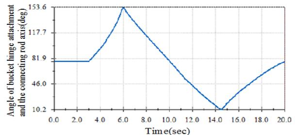
Fig.8. The changing angle of bucket hinge attachment and the connecting rod axis
