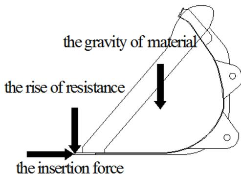
Fig.3. Force loading location
