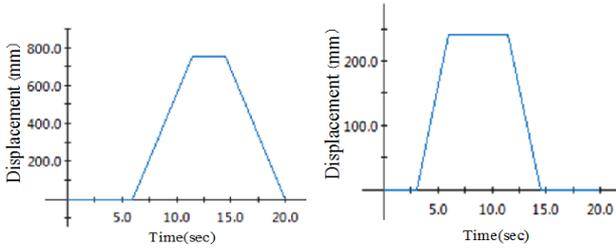
Fig.2. The curves of displacement for lifting cylinder and tilting cylinder
