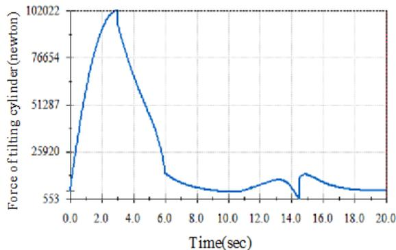
Fig.10. The changing force of tilting cylinder
