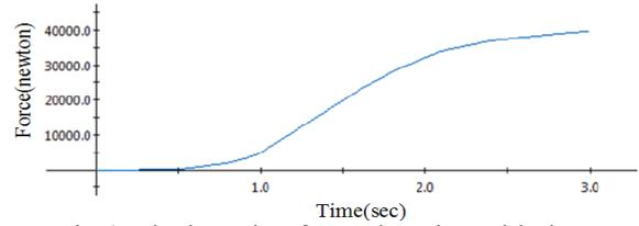
Fig.4. The insertion force changing with time
