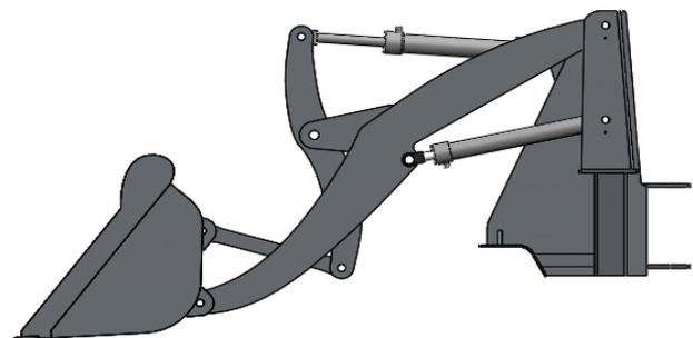
Fig.1. Three-dimensional working equipment of loader assembly model
