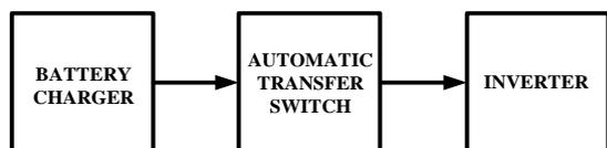
Fig.1. Basic units of the multi-powered UPS
