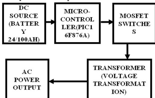
Fig. 2: Components of the Inverter
