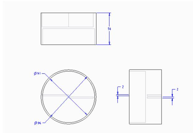
Fig.7. Part drawing of rotating ring
