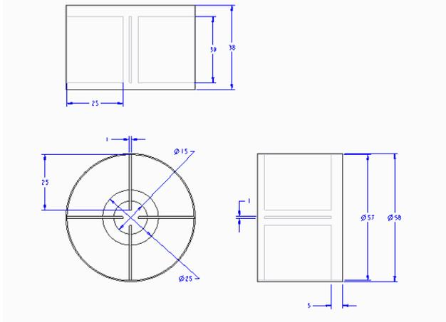
Fig.9. Part drawing of base holder
