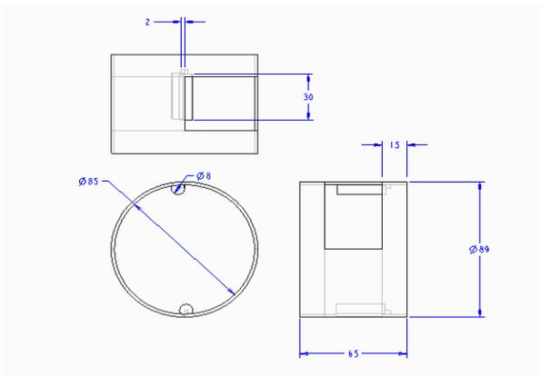
Fig.5. Part drawing of blade holder
