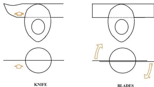
Fig.13. cutting with knife on left and with new system right
