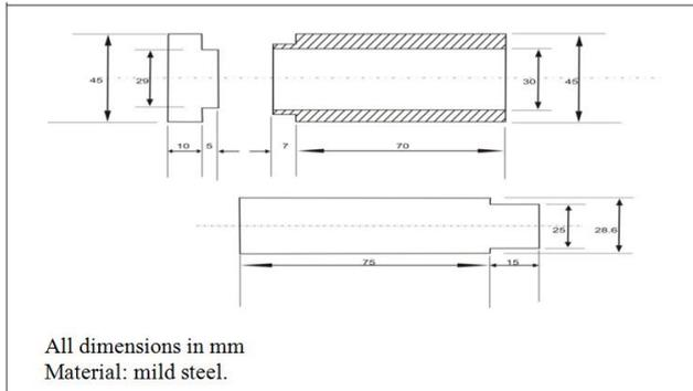
Fig. 1. Cylindrical Steel mould
