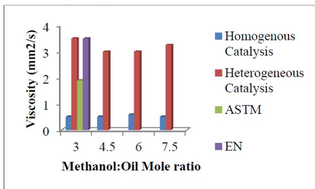
Fig.4. Comparison of viscosities of products with International Standards
