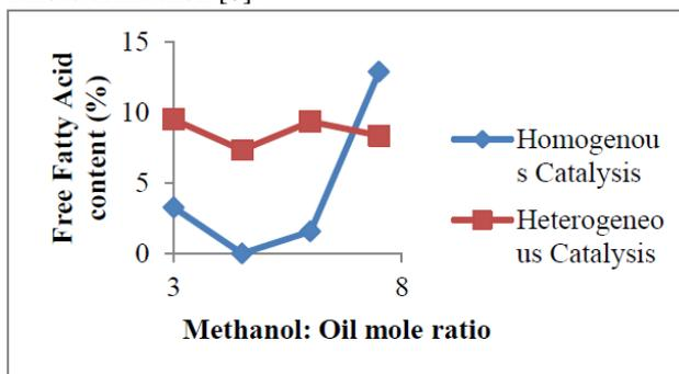
Fig.2. Comparison of free fatty acid content in the products
