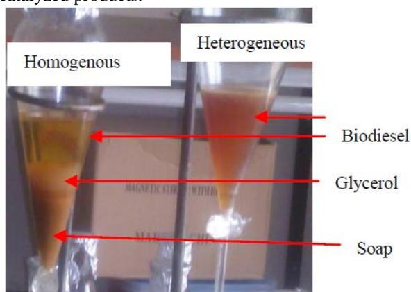
Plate 1: The two products of the transesterifications in separation process
