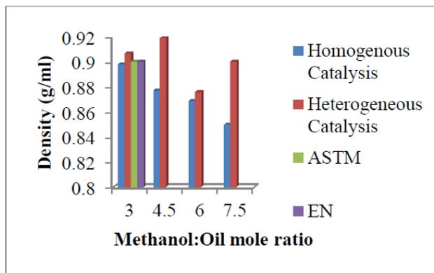
Fig.5. Comparison of densities of products with International Standards
