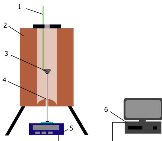
Fig.2. Schematic chart of measuring device: 1 – holder for inserted sample; 2 – hot-air oven; 3 – crucible with tested sample, 4 – interconnecting rod; 5 – scales; 6 – computer [10, 11]
