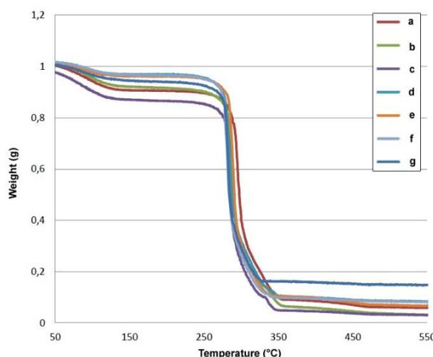
Fig.3. Thermogravimetric curves of measured samples
