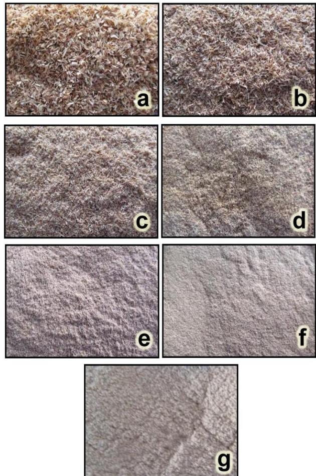
Fig.1. Samples of individual fractions of the wood dust: a = 1 000  $\mu\text{m}$  – 2 500  $\mu\text{m}$ ; b = 500  $\mu\text{m}$  – 1 000  $\mu\text{m}$ ; c = 250  $\mu\text{m}$  – 500  $\mu\text{m}$ ; d = 200  $\mu\text{m}$  – 250  $\mu\text{m}$ ; e = 150  $\mu\text{m}$  – 200  $\mu\text{m}$ ; f = 71  $\mu\text{m}$  – 150  $\mu\text{m}$ ; g = 0  $\mu\text{m}$  – 71  $\mu\text{m}$
