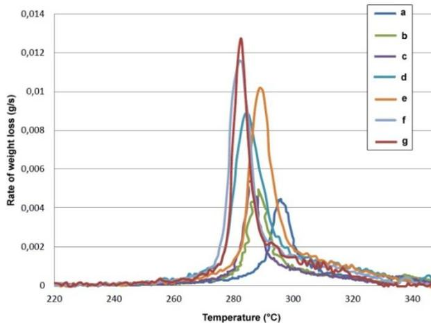
Fig.5. Derivative thermo-gravimetric curves of tested samples
