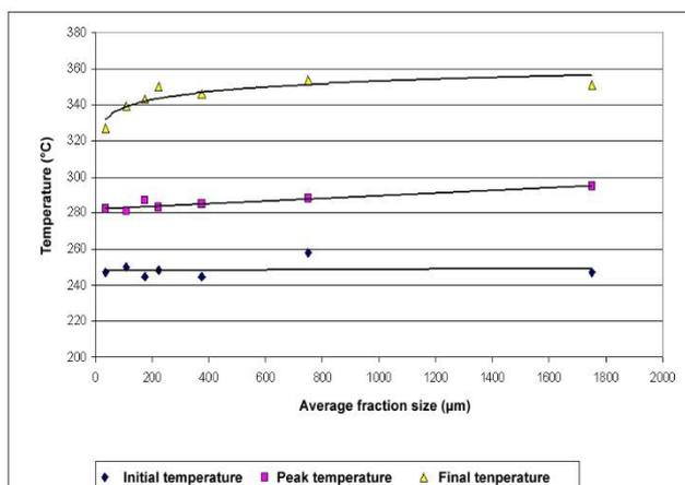
Fig.6. Dependence of initial, peak and final decomposition temperature of wood dust on average fraction size
