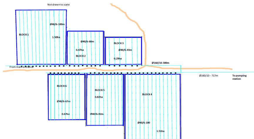
Fig.I. Sprinkler Irrigation Design for Aiyinase Station (not drawn to scale)
