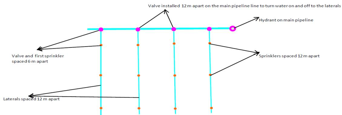
Fig.II. Schematic layout of sprinkler systems
