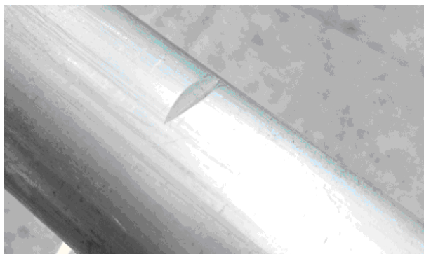
Fig. 2. A picture of the local sharp-cut circular tube.
