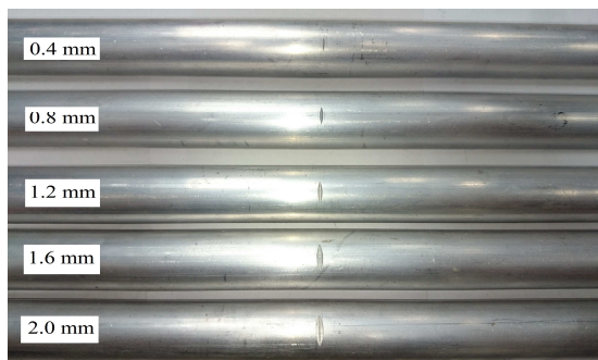
Fig. 6. Picture of the tested 6061-T6 aluminum alloy circular tubes with different cut depths.
