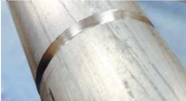
Fig. 1. A picture of the circumferential sharp-notched circular tube.
