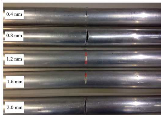
Fig. 14. A picture of the failure for local sharp-cut 6061-T6 aluminum alloy circular tubes with a = 0.4, 0.8, 1.2, 1.6 and 2.0 mm under cyclic bending.
