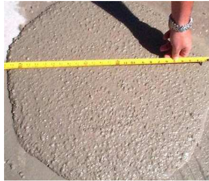
Fig. 2. Slump Test Result for grade 50 (G50) SCC sample
