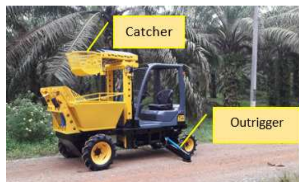
Fig. 7. Interesting part of mobile bunch catcher
