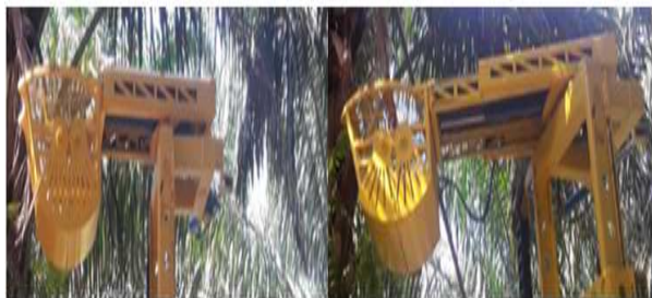
Fig. 12. Left: catcher in shortest arm and right: catcher in longest arm
