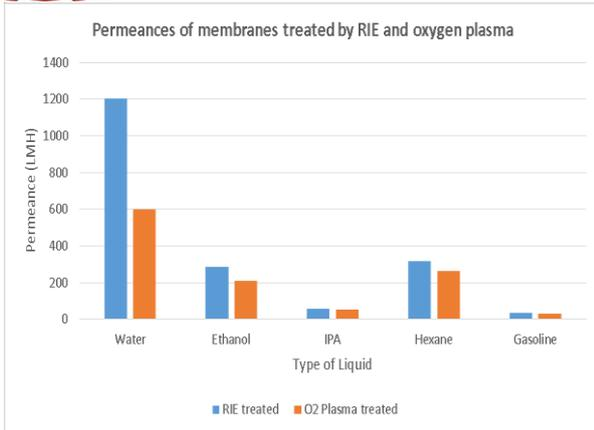
**Figure 10.** Permeance of RIE-treated PDMS-based (blue bars) and Oxygen-plasma-treated Polystyrene-based (orange bars) VACNT membranes, for various polar and non-polar liquids.
