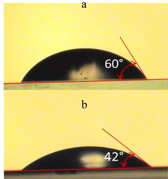
**Figure 9.** Photographs of a water drop on the VACNT membrane a) before RIE etching and b) after RIE etching. Contact angle decreases from  $60^\circ$  before etching to  $42^\circ$  after etching.
