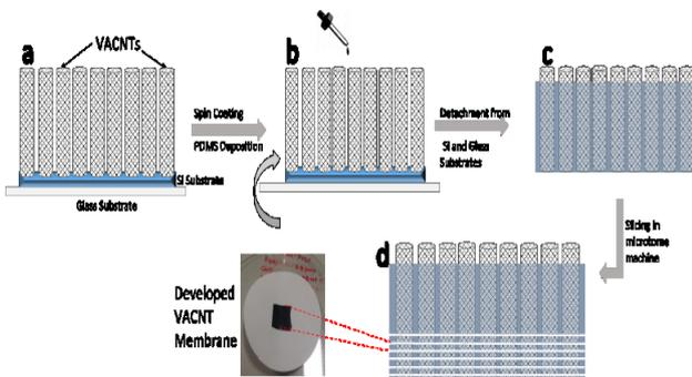
Figure 2. VACNT membrane fabrication process. a) VACNT on silicon substrate glued to glass. b) PDMS addition and spin coating. c) After drying, silicon and glass substrates are detached using mechanical peeling. d) VACNT-PDMS composite is sliced using a microtome machine [14].
