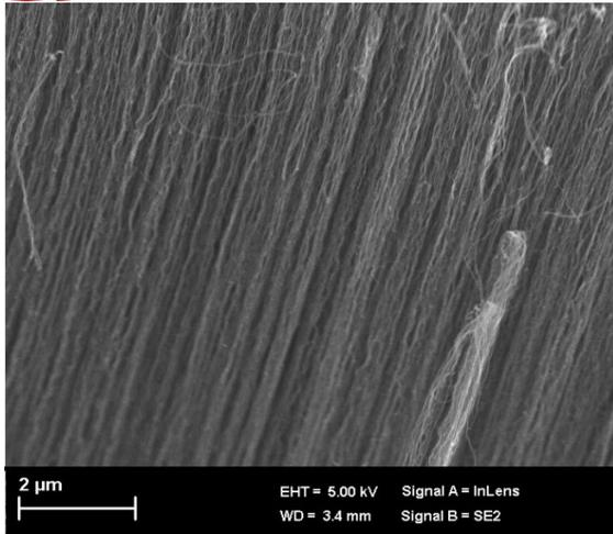
Figure 1. Cross section of the developed VACNT array.
