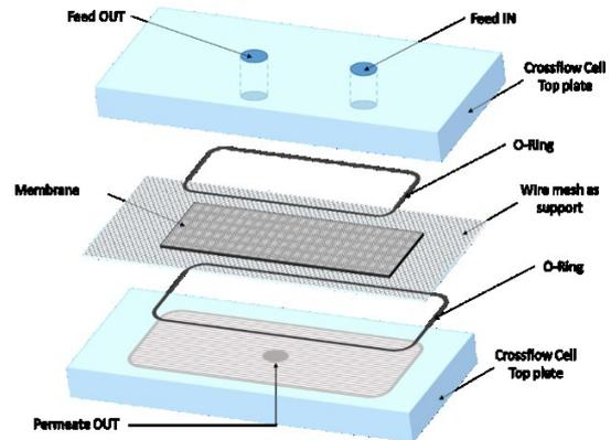
Figure 3. Schematic of the developed crossflow cell. The VACNT membrane is placed on a wire mesh support and sandwiched between acrylic plates before sealing the cell with O-rings to enable feed filtration at high pressure.
