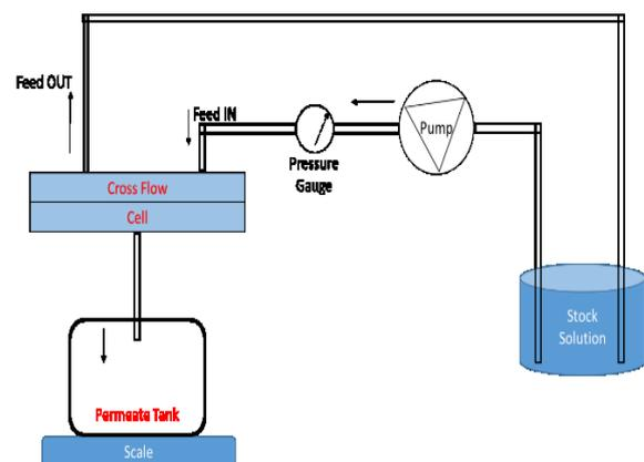
Figure 4. Benchtop crossflow setup used to investigate the performance of the developed VACNT membranes.
