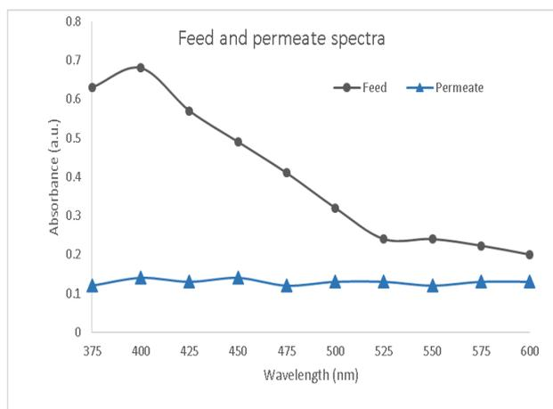
Figure 6. UV-Vis spectra of the iron oxide solution at the feed side and the collected permeate [14].
