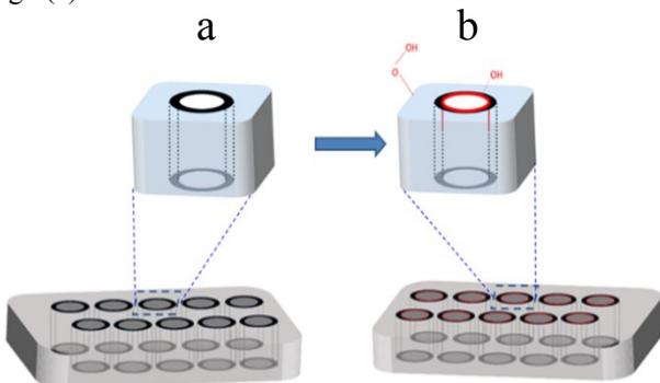
**Figure 8.** a) Hole opening after dry etching (RIE). b) Illustration of the formation of hydroxyl ion on PDMS and VACNT entrance. The black rings represent MWCNTs, whereas the dotted line connecting the black rings between the top to bottom surfaces of the membrane are just a depiction of the vertical alignment of the CNTs.
