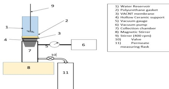
Figure 5. Modified dead-end cell setup used to measure the VACNT membrane performance [14].
