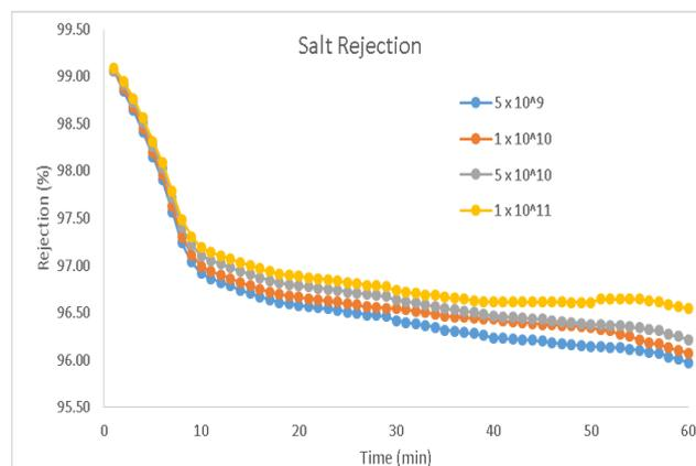
Figure 7. This is extracted graph of the Salt rejection versus time, for the different developed VACNT membranes [14].
