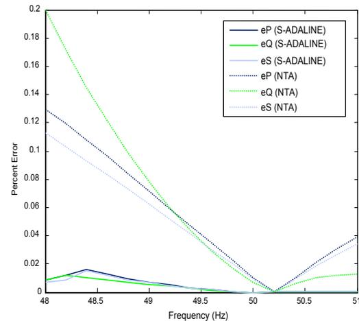
**Figure 5:** Absolute %errors in power components estimation under off-nominal frequency
