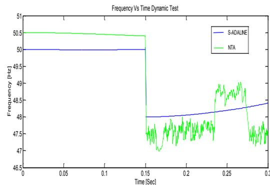
**Figure 6:** Estimated Frequency Comparison of NTA and proposed S-ADALINE
