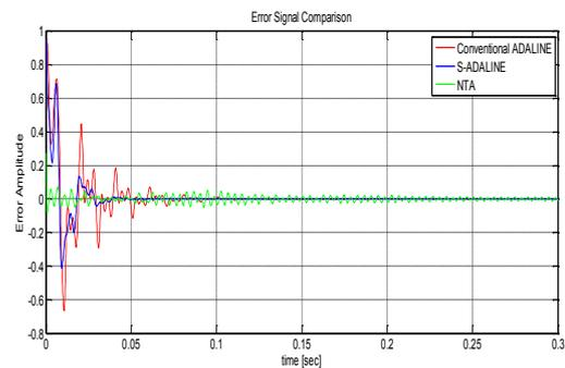
Figure 3: Error Comparison of Conventional ADALINE, NTA and proposed S-ADALINE at Nominal frequency condition (50 Hz)
