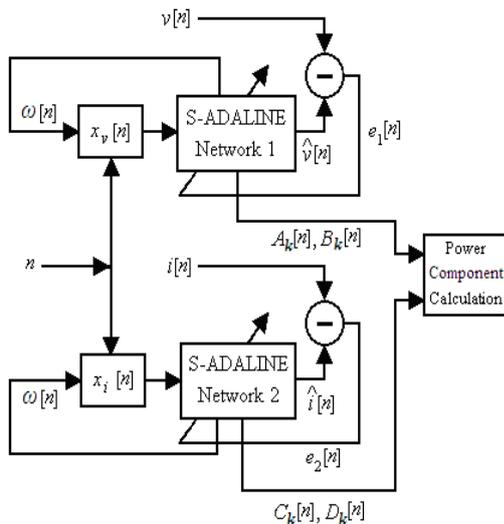
Figure 2: Block diagram of S-ADALINE based power component measurement unit
