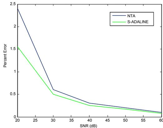
**Figure 7:** Absolute maximum steady-state errors in active power estimation in terms of SNR
