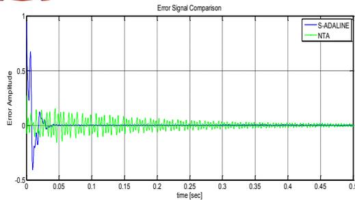
**Figure 4:** Error Comparison of Conventional ADALINE, NTA and proposed S-ADALINE at Off-nominal frequency condition (48 Hz)
