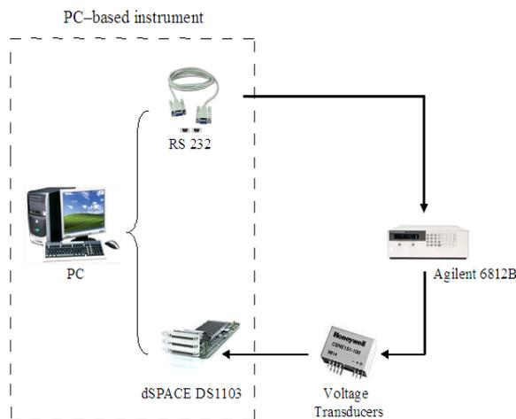
**Figure 8:** Laboratory test setup for the amplitude tracking
