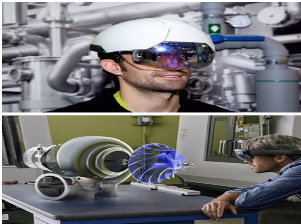
Fig. 2. Head mount display with augmented reality
