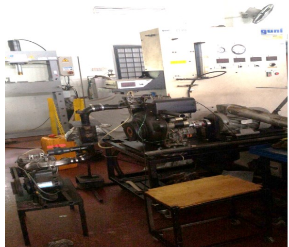
Fig. 3: Engine test rig based on GUNT asynchronous dynamometer
