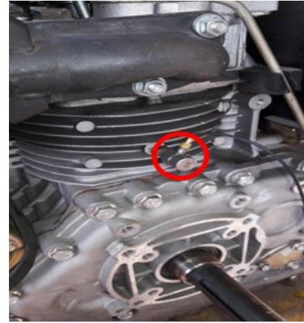
Fig. 6. Accelerometer sensor mounting
