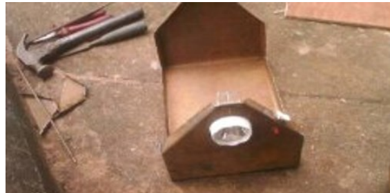
Fig. 2. Machine bed construction of a prototype inflator.
