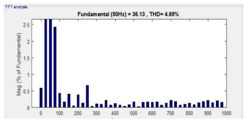
Fig. 5. Frequency analysis of source current waveform for balanced load shown 4.69% THD.
