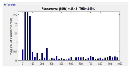
Fig. 7. Frequency analysis of compensated source current for unbalanced load shown 4.69% THD.
