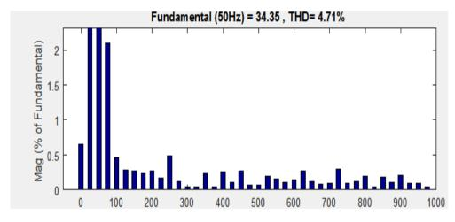
Fig. 9. Frequency analysis of source current waveform for balanced load shown 4.71% THD.
