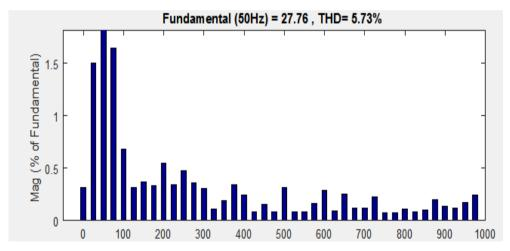
Fig. 11. Frequency analysis of compensated source current for unbalanced load shown 5.73% THD.
