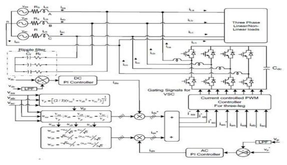
Fig. 2. Diagram of Vsc based Dstatcom with Hysteresis current control technique.
