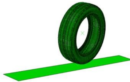
Fig. 1. Finite element model of tire.
