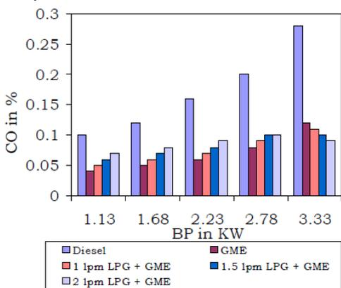
Fig. 8. CO emissions of Diesel, GME and its blends with LPG
