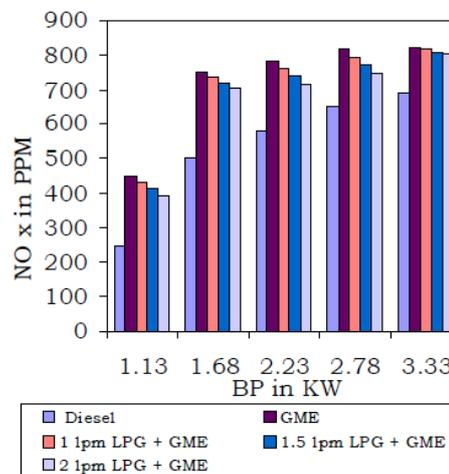
Fig. 9. NOx emissions of Diesel, GME and its blends with LPG
