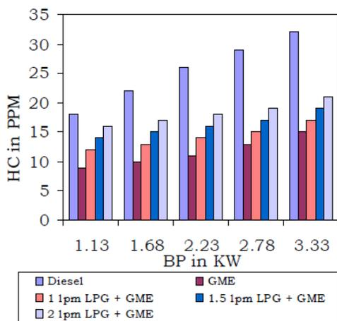
Fig. 7. HC emissions of Diesel, GME and its blends with LPG
