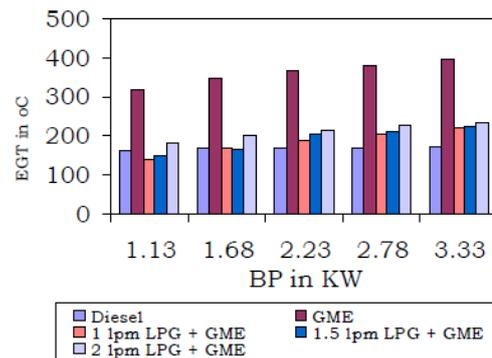
Fig. 7. Exhaust Temperature of Diesel, GME and its blends with LPG
