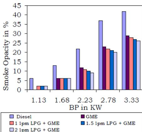
Fig. 10. Smoke emissions of Diesel, GME and its blends with LPG
