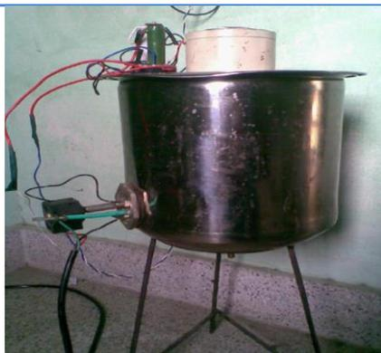
Fig. 1. Shows Transesterification reactor
