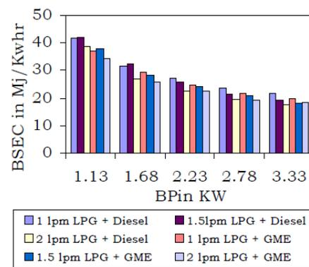
Fig. 6. Brake Specific Energy Consumption Diesel blend with LPG and GME blend with LPG
