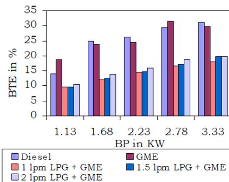
Fig. 5. Brake Thermal Efficiency of GME and its blends with LPG
