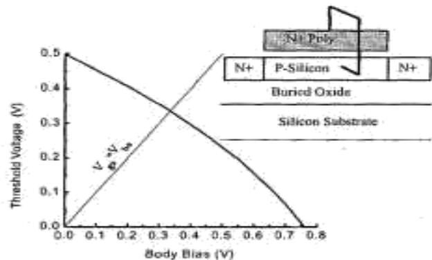
Fig. 3. DTMOS NFET and threshold-voltage variation curve
