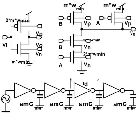
Fig. 6. DT MOS Circuit configurations for simulations. The FB-CMOS gates have the same topology minus the body contacts
