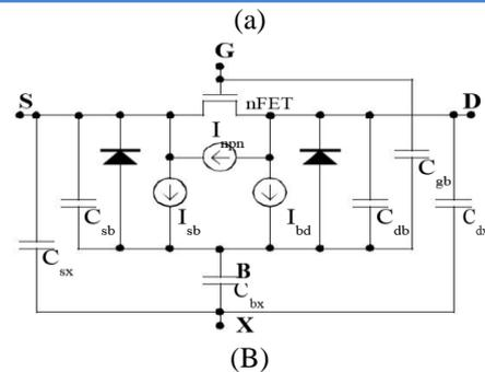
Fig. 2. (a) Schematic cross section of a PD-SOI nFET. (b) Equivalent circuit model. ( $I_{npn}$  is the parasitic lateral npn current, the diodes are the base-emitter and base-collector junction diodes,  $I_{sb}$  and  $I_{bd}$  are impact ionization currents.) [3]
