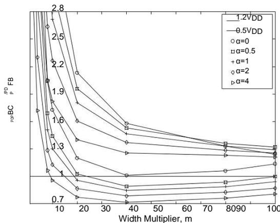
Fig. 7. Normalized FO1 inverter delay and power for various wire loads
