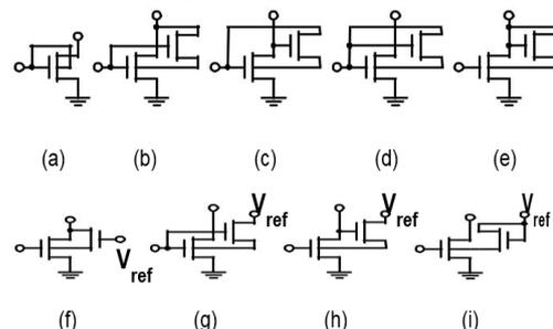
Fig. 1. DTMOS circuit configurations in the literature.
