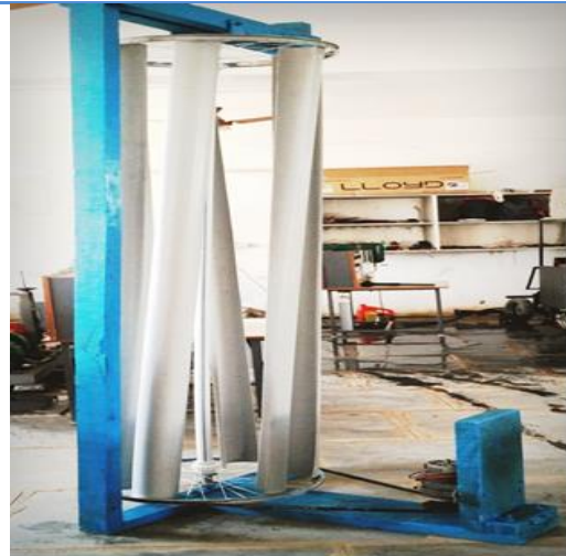
Experimental setup vertical axis wind turbine.
