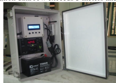
Fig.4. Module of Monitoring Station.
