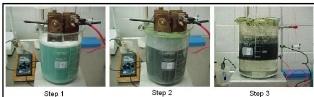
Fig.6. Aspect of the three stages (early, after 15 minutes and the separation of the phases) of the electrolytic treatment of batch standard sample "B".
