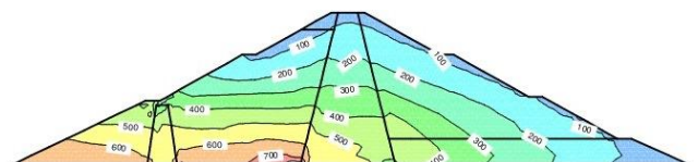
Fig.10. Horizontal stress distribution at the end of first impounding
