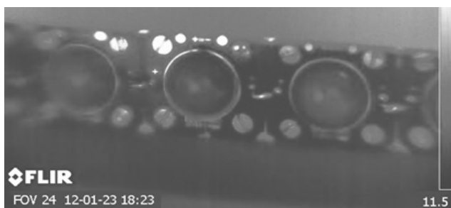
Fig.1. An infrared view of tested LEDM and LED
