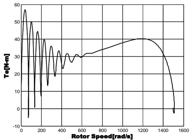
Fig.5: Electromagnetic Torque against Mechanical Rotor Speed
