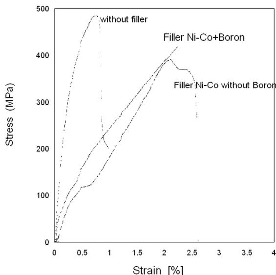
Fig.4. Tension tests plots of the samples without filler material (blade material), welded samples with Ni-Co and Ni-Co boron doped alloys.
