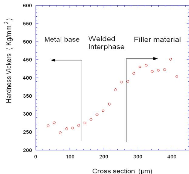
Fig.3. Hardness Vickers profile along the: base material-HAZ-filler material.
