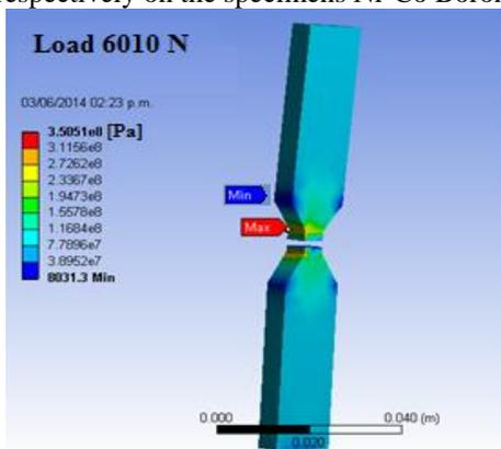
Fig.7a. Schematic representation of the maximum and minimum stresses in sample boron doped.
