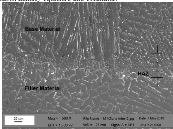
Fig.2. Inter-phase of the Heat affected Zone (HAZ) and filler material
