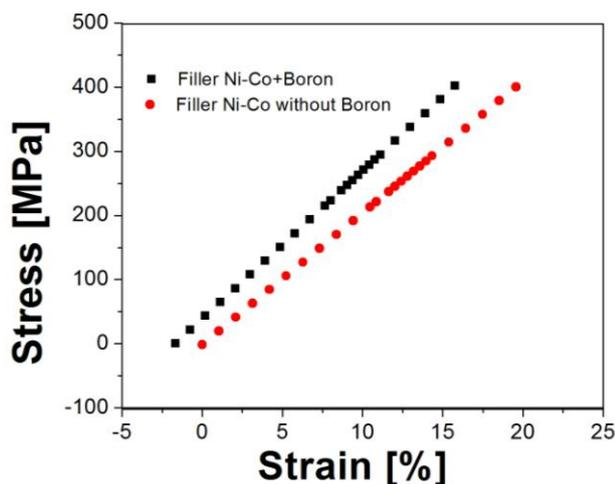
Fig. 9. Numerical representations of the stress-strain curve for samples in the elastic zone.
