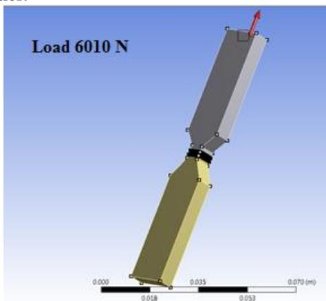
Fig.6b. Schematic representation of the applied stress direction with a load of 6010N.
