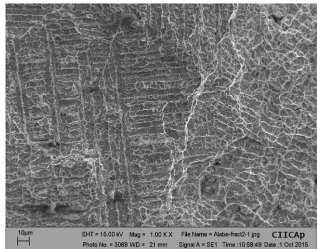
Fig.5b. Fracture surface of the Ni-Co boron doped sample exhibiting ductile dimple morphology.
