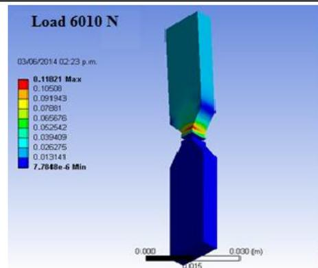
Fig.7b. Schematic representation of the maximum and minimum strains in sample boron doped.
