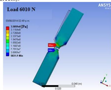
Fig.8a. Schematic representation of the maximum and minimum stresses in sample without boron additions.
