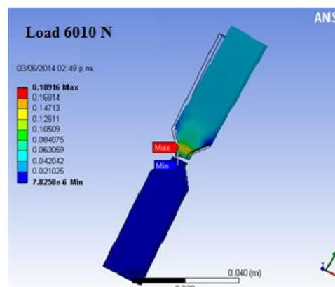
Fig.8b. Schematic representation of the maximum and minimum strains in sample without boron additions.
