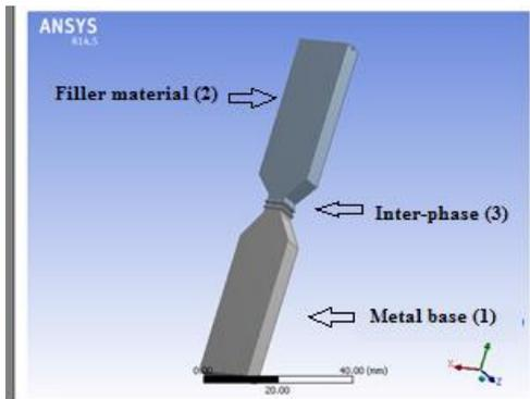
Fig.6a. Schematic representation of Metal base (1), Filler material (2) Inter-phase (3)
