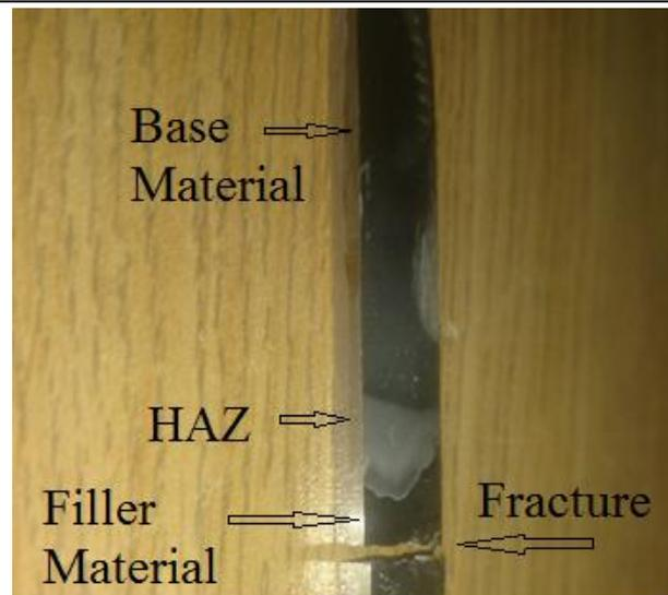
Fig.5a. Fractured sample after the tension test, showing that failure occurs on the filler material and not in the HAZ interphase.
