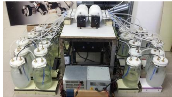
Fig.1. Apparatus constructed for the indirect biodegradability measurement.
