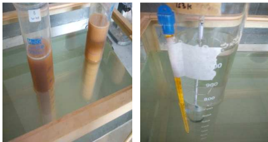
Fig. 2. Sedimentation test by hydrometer in water bath
