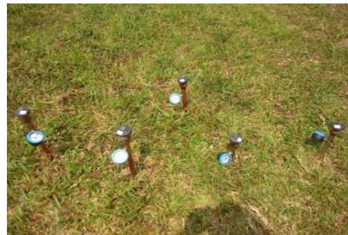
Fig. 3. Field monitoring at different depths by tensiometers at the study area
