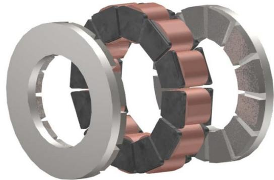
Fig. 1. Axial-flux PM machine with segmented stator topology [16]
