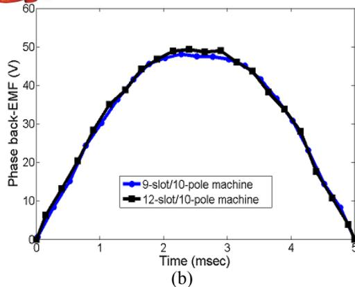
**Fig. 5.** (a) flux linkage waveforms by 3-D FE transient simulation (b) back-EMF waveforms by 3-D FE transient simulation
