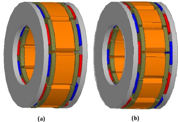
**Fig. 2.** Similar pole and slot combination. (a) 9-slot/10-pole axial-flux motor (b) 12-slot/10-pole axial-flux motor
