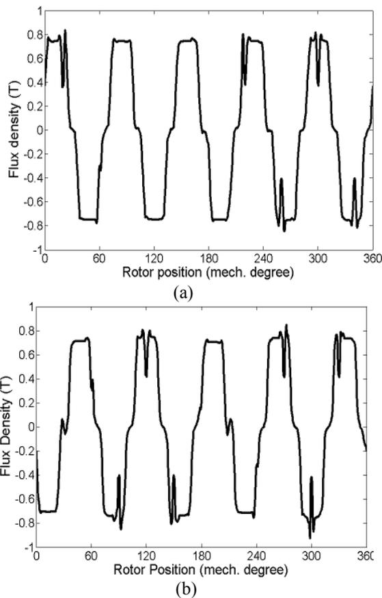
**Fig. 3.** 3-D FE flux density waveforms for (a) 9-slot/10-pole machine (b) 12-slot/10-pole machine
