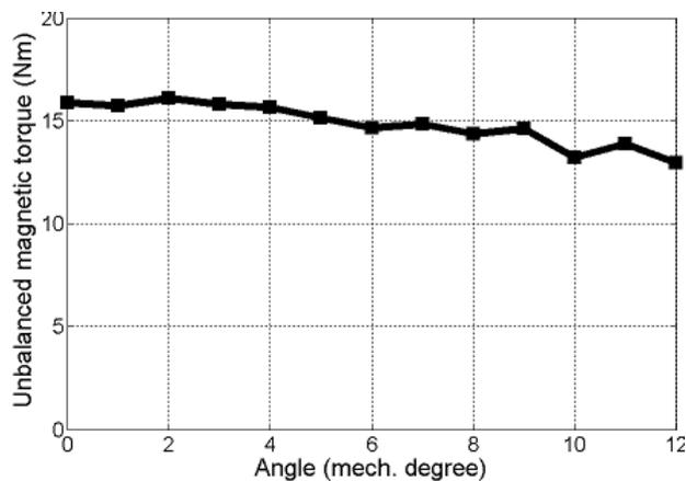
**Fig. 6.** 3-D FE unbalanced torque exerted on bearing in 9-slot/10-pole machine
