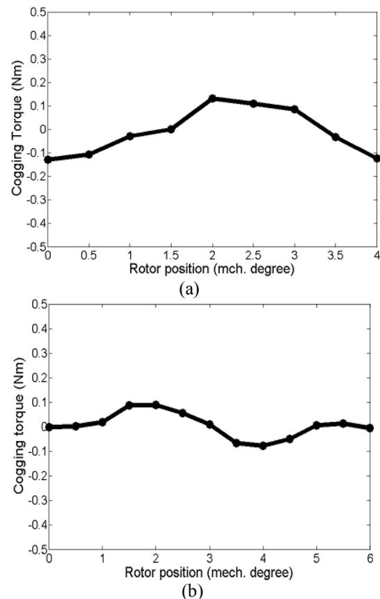
**Fig. 4.** 3-D FE cogging torque waveforms for (a) 9-slot/10-pole machine (b) 12-slot/10-pole machine
