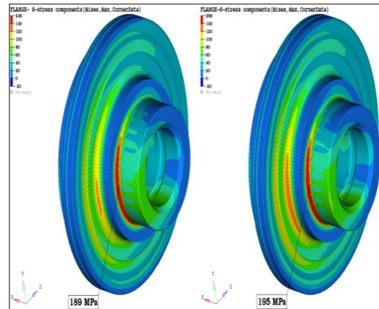
**Figure 11:** Von-Mises stress Results for Flange
