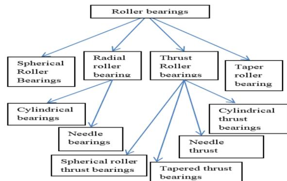
Figure 1: Classification of Roller Bearings
