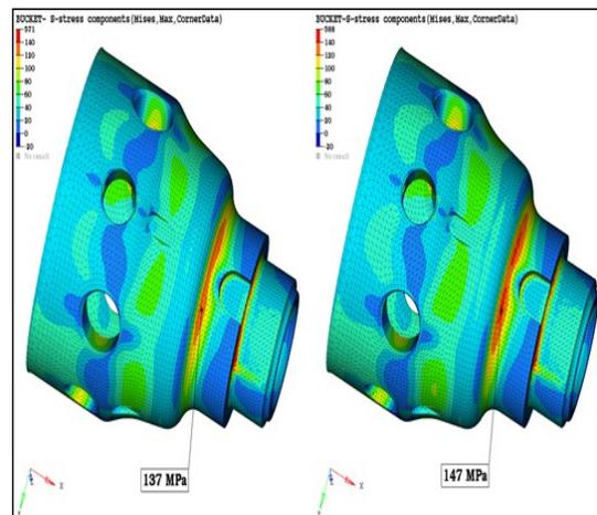
**Figure 12:** Von-Mises Stress results for Bucket
