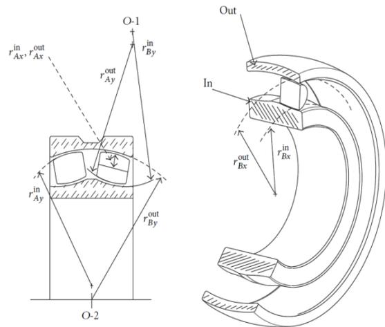
**Figure 2:** Radii of curvature between roller, inner race and outer race
