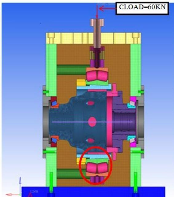
**Figure 10:** Schematic of the differential bucket test set-up with the loading conditions and boundary shown. The location circled red is where the SRB sits.
