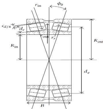
Figure 3: Dimension of Spherical Roller Bearing
