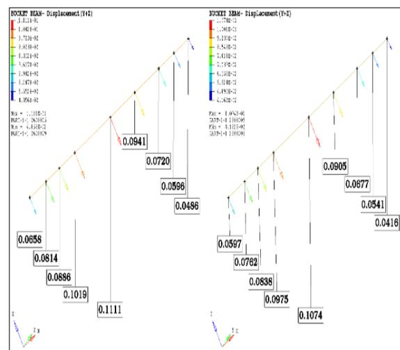
**Figure 13:** Bending Displacement values at Different node Positions of Bucket Beam Element
