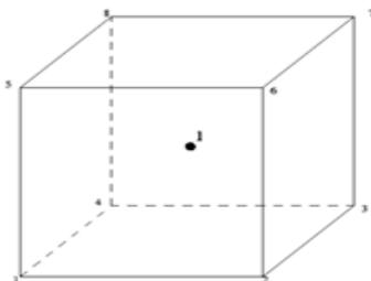
**Figure 6:** Integration Point Scheme in C3D8R Element
