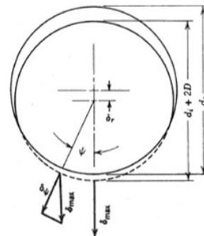
Figure 4: Radial Displacement of SRB
