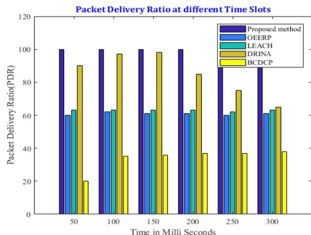
Fig. 4. Packet delivery ratio at different time slots
