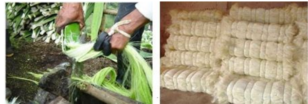
Fig. 1. Sisal fibers extraction and fibre bundles
