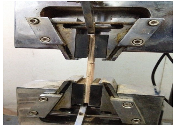
Title 5: Glue shear strength. Plate 5: Fixing the sample in UTM for testing
