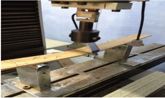
Title 6: Bending Strength Test Plate 6: Application of load during test.
