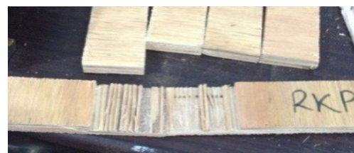
Title 8: Glue shear strength test. Plate 8: wood failure.
