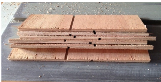
Title 4: sampling. Plate 4: Preparation of Glue shear strength samples.
