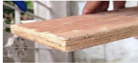
Title 7: Water resistance test. Plate 7: check for delamination.
