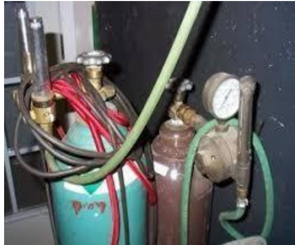
Fig. 2. Shielding Gas (P.C. Okolie et al, 2019).
