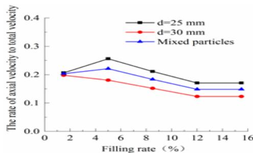
Fig. 13. Filling rate affect the two-component particles' rate of axial velocity to total velocity.
