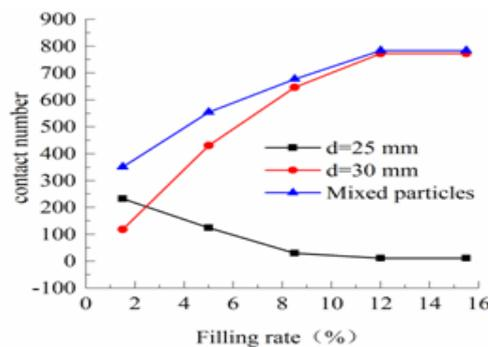
Fig. 14. Filling rate affect the number of two-component particles in contact with the wall.
