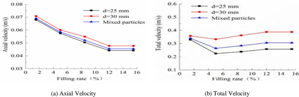
Fig. 12. Filling rate affect the two-component particles axial velocity and total velocity.
