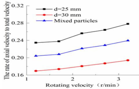
Fig. 10. Rotating velocity affect the two-component particles' rate of axial velocity to total velocity.
