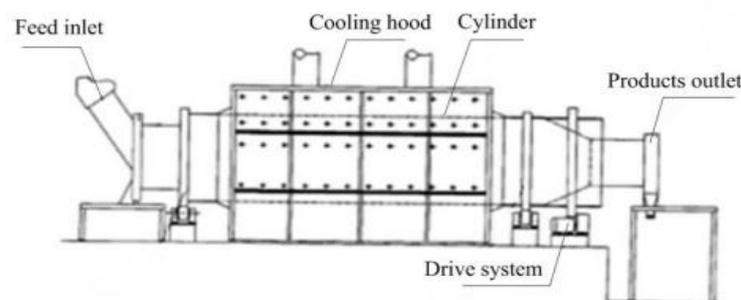
Fig. 1 Sketch map of the drum cooler structure.
