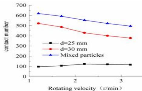
Fig. 11. Rotating velocity affect the number of two-component particles in contact with the wall.
