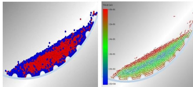
Fig. 5. Two-component particles bed morphology and velocity vector cloud image.
