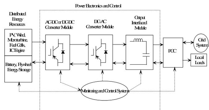
Fig.1 General Purpose block diagram of DG-grid system.
