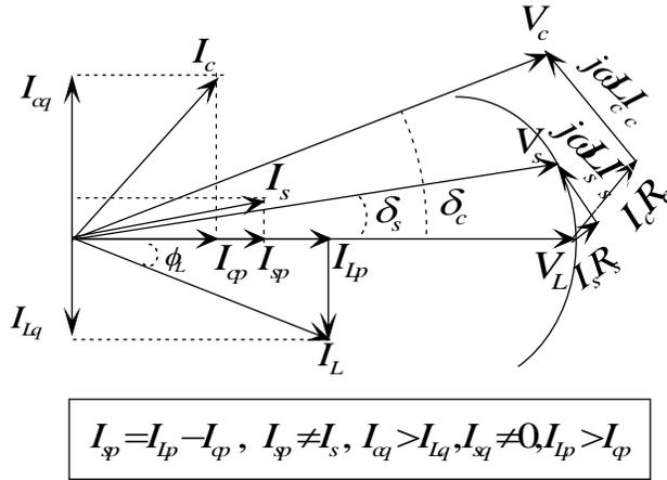
Fig.6. Phasor diagram at zero voltage regulation in forward interconnected mode.
