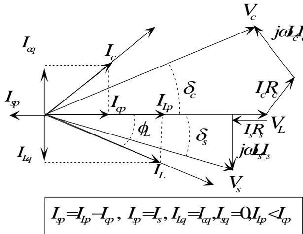
Fig.7. Phasor diagram at unity power factor in reverse interconnected mode.
