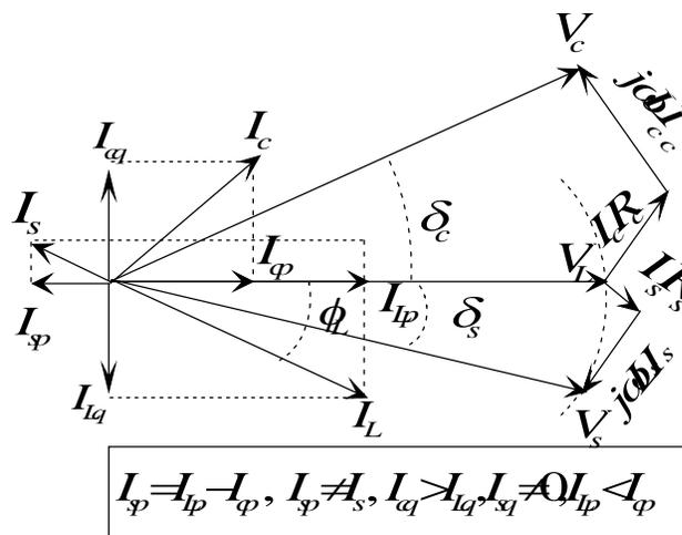
Fig. 8. Phasor diagram at zero voltage regulation in reverse interconnected mode.
