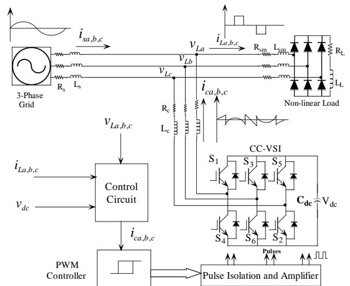
Fig.2. Topology of shunt active power filter.
