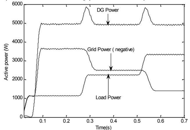
Fig.13. Grid, load and DG active powers in reverse interconnected mode of operation.
