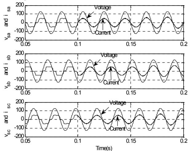
Fig. 10. Grid voltages and currents before and after compensation without DG.
