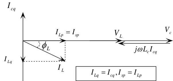
Fig. 9. Reactive power control (The grid alone is supplying total power to load).
