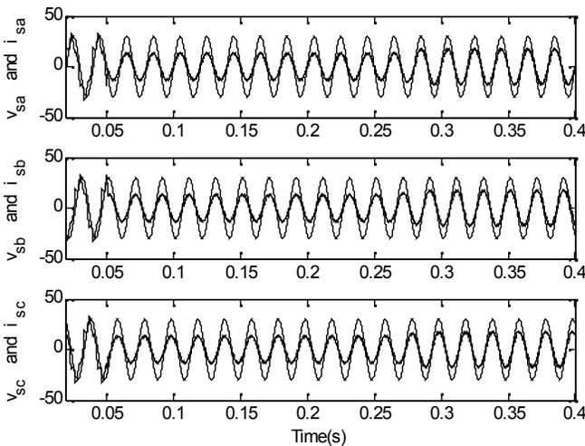
Fig. 12. Three-phase grid voltages (scaled by a factor of 0.1) and currents in forward interconnected mode.
