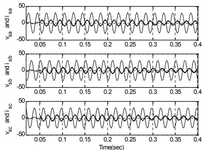
Fig. 14. Three-phase grid voltages (scaled by a factor of 0.1) and currents in reverse interconnected mode.
