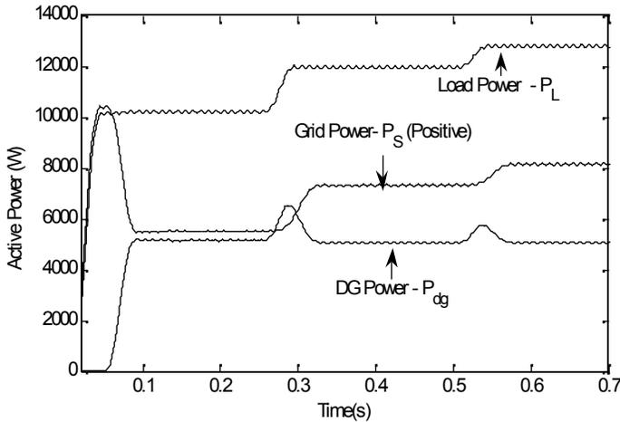
Fig.11. Grid, load and DG active powers in forward interconnected mode of operation.
