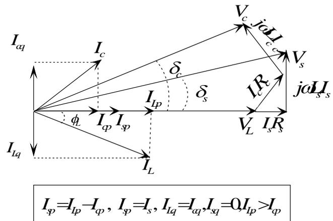
Fig.5. Phasor diagram at unity power factor in forward interconnected mode.
