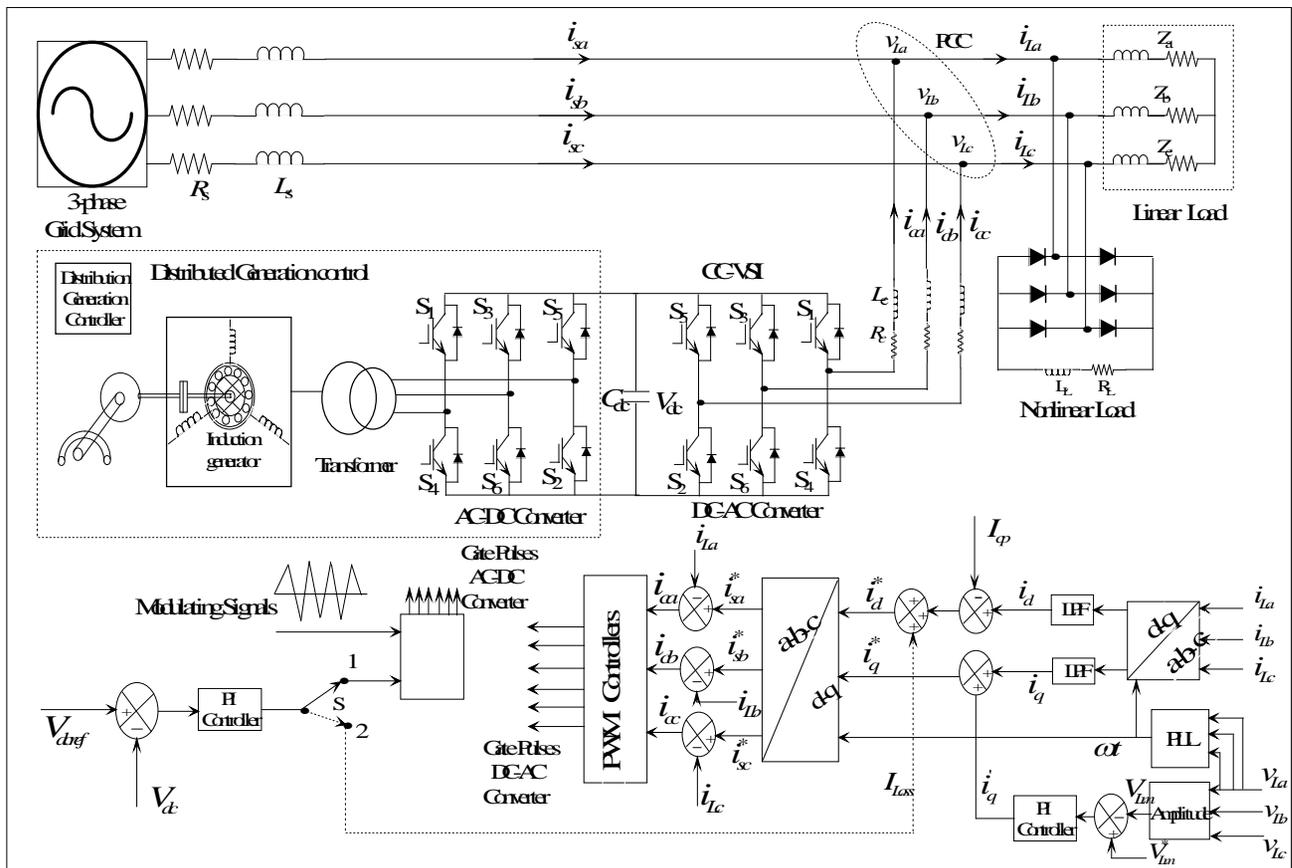
Fig.4. Schematic diagram of power and control circuit of the proposed DG-Grid system interfaced with active power filter.
