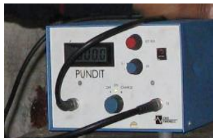
Fig.3. Portable Ultrasound Non-destructive Digital Indicator Tester Equipment (PUNDIT)
