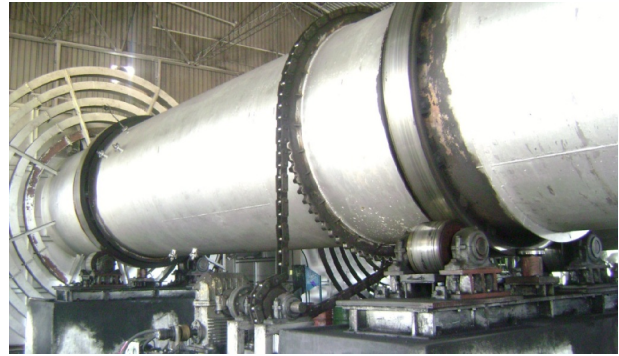
Fig.1. Rotary kiln arrangement
